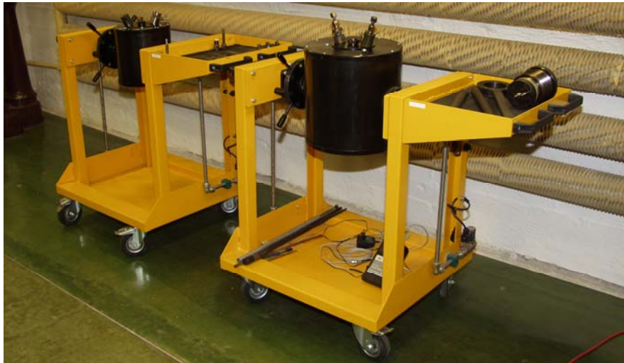
Picture 17. Experimental stands with 200 cm 3 and 700 cm 3 closed vessels for determining energy and ballistic characteristics of solid propellants
