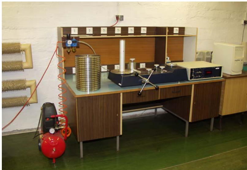
Picture 19. Experimental set-up for static calibration of piezoelectric pressure transducers
