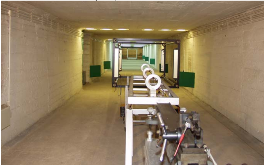
Picture 8 Firing indoor range in the Ballistics Laboratory with the apparatus measuring ballistic characteristics of weapons and ammunition
