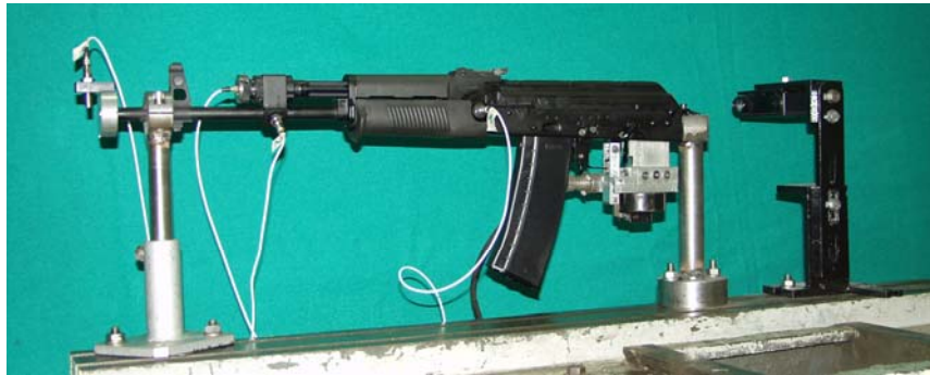
Picture 16. Experimental stand type 5,56B to test weapon dynamic characteristics and gas port
