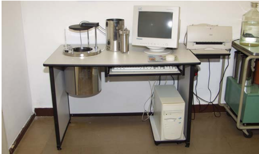
Picture 18. Experimental stand for determining the combustion heat of solid throwing and propelling materials
