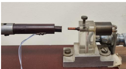
Fig.13. Mutual position of the coils on the laboratory stand: a) no coupling, b) maximum coupling.
