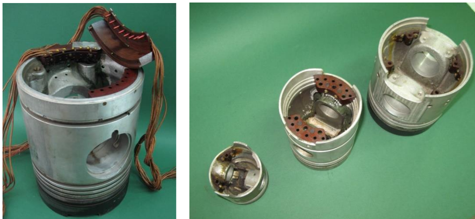
Fig. 7 Pistons of 8C22, PF 125p, Leyland SW680 and Wola H6 engines prepared for temperature measurements
