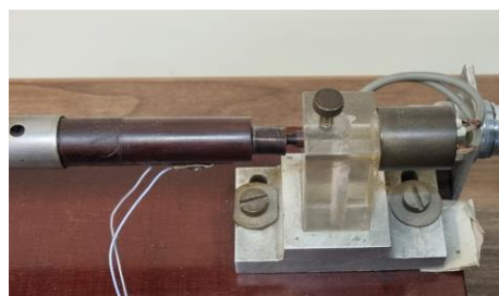
Fig.13. Mutual position of the coils on the laboratory stand: a) no coupling, b) maximum coupling.
