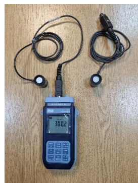
Rys. 7 Foto-Radiometer HD-2102.2 with LP 471 – PHOT probe. LP 471-RAD probe for measuring heat flux density lies next to it.
