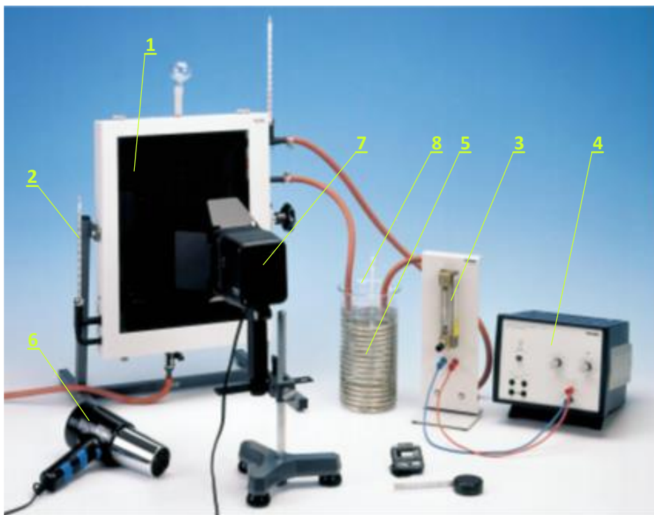
Fig. 3 Main components of a flat plate solar collector test stand [1, 2]
