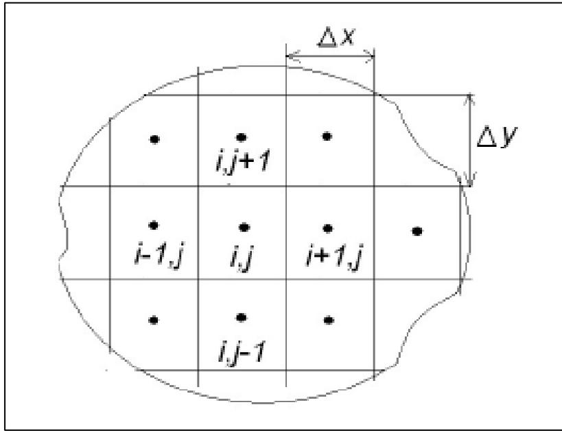
**Fig. 1.** Example of the discretization area using the finite difference method.
