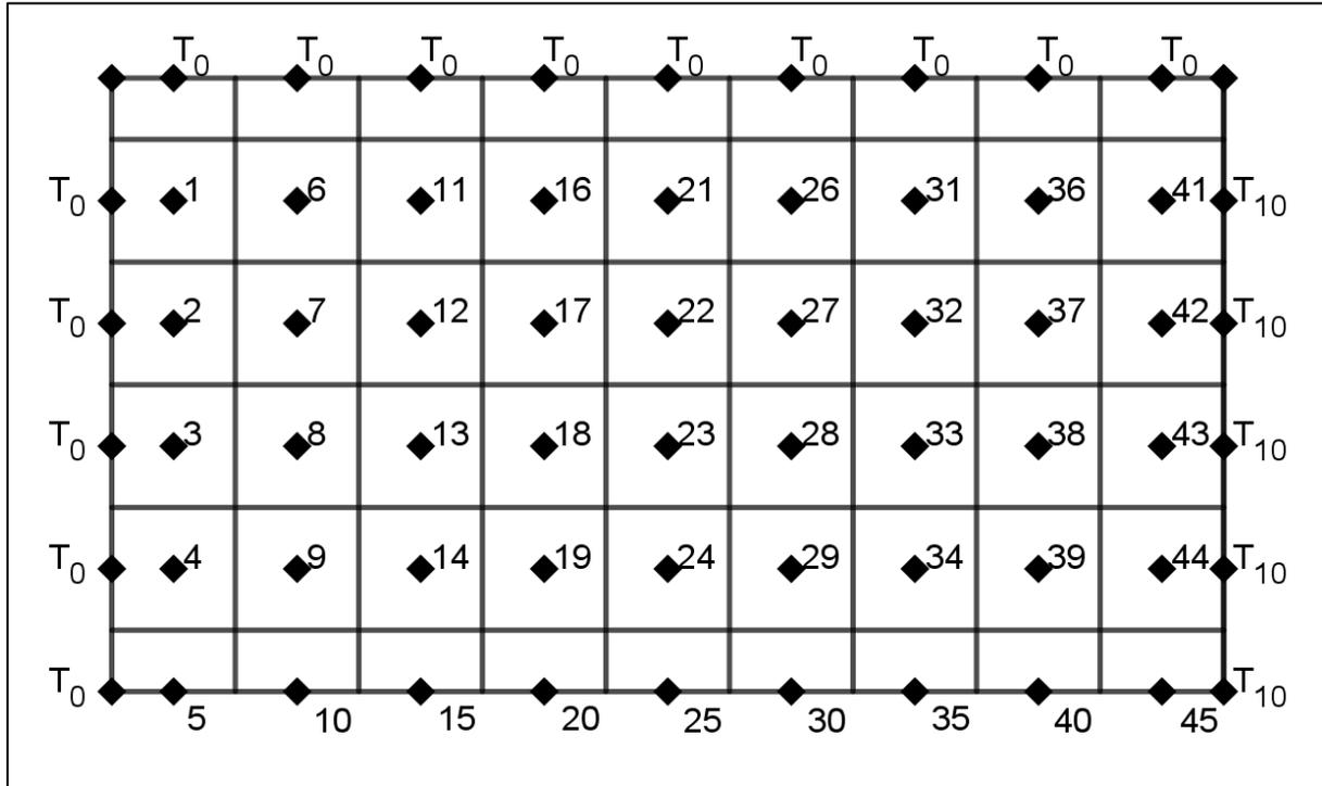
Fig. 9. Discretization of half of the square area and numbering with a discretization step of 0.1π
