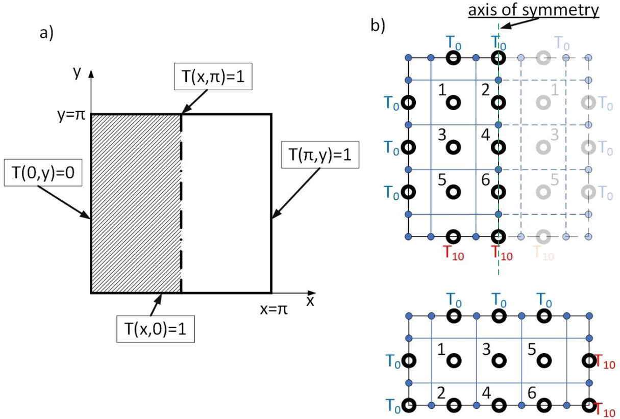
Fig. 2. a) Square plate heated along one side, b) discretization of half of the square area and node numbering with a discretization step of  $\pi/4$
