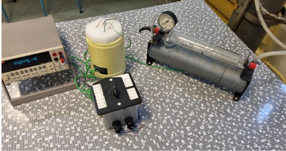
Fig.3 Laboratory stand for testing the Joule-Thomson effect
